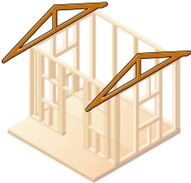
Figure #10 Gable Truss Installation
