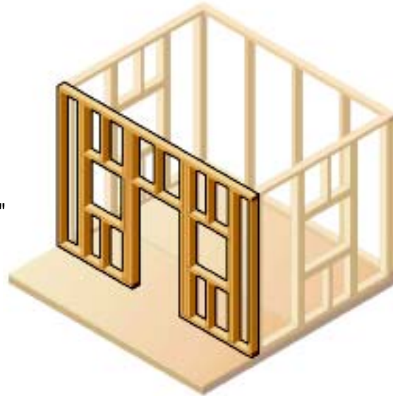
Figure #8 Front And Back Wall Installation
